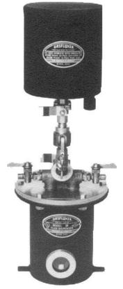
A neddle valve regulates the amount of Gasflux carried to the torch by directing all or only part of the fuel gas into the Gasfluxer mixing chamber. Once the valve is set for the required amount of flux needed, the Gasflux process becomes automatic.
